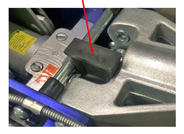
Insert round jack handle into mechanism and push down firmly. Remove plastic insert.
